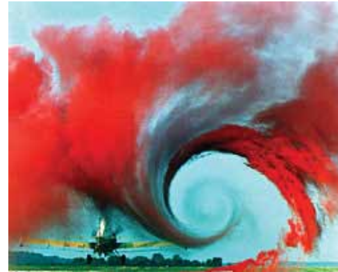
The vortex in the wake of an airplane
